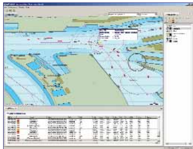
Port of Hamburg with some real situation tracking of civil vessels via AIS (Automatic Identification System). Tabel below shows additional information on each vessel
