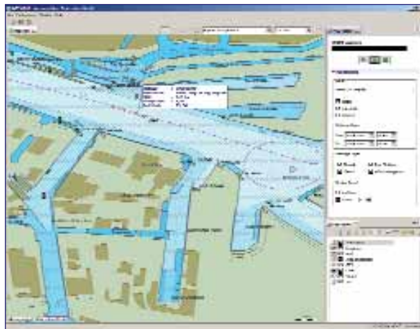
AGIS 4000 can replay the complete AIS traffic for a specified period of time. The replay creates a new layer in the map view. The user can also choose the replay speed (real-time or multiplied by a factor)
